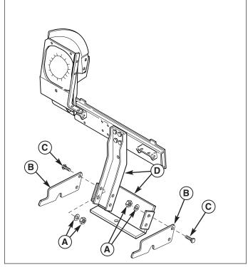
Figure 7. Assemble Catcher Frame (Prestige Shown)
